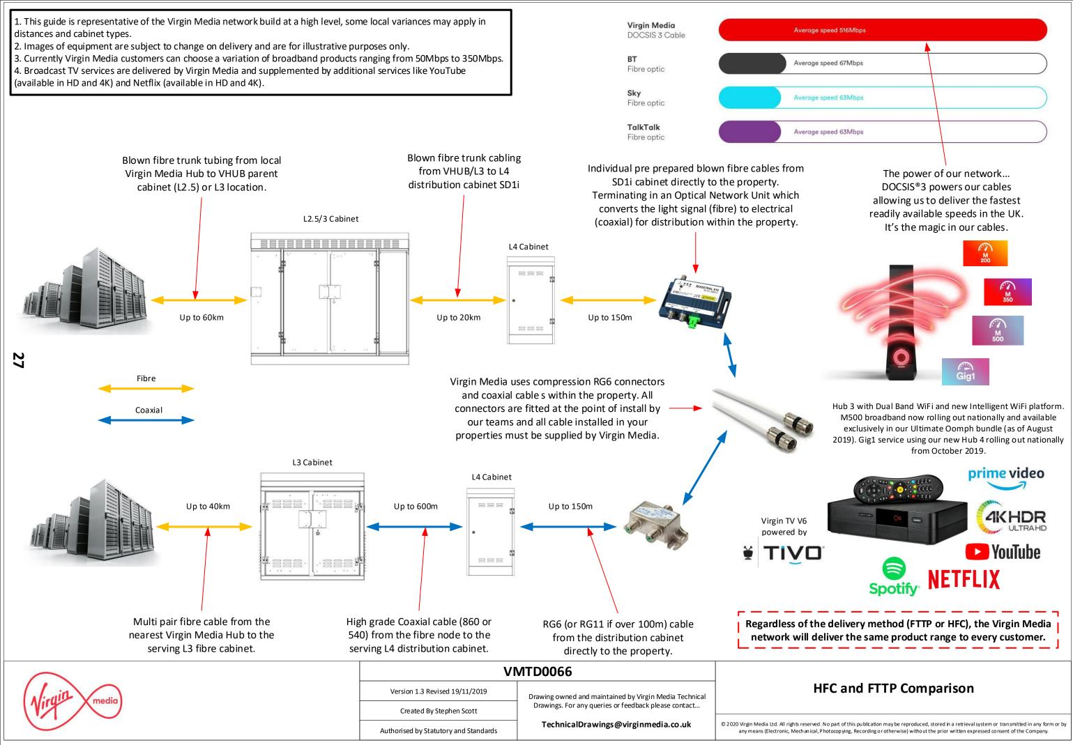
Currently our FTTP Omni box can support up to 4 internal points, each internal point will consist of a single RG6 coaxial cable terminated back to the Omni box. Power for the ONU is supplied through a power inserter connected to one cable from the primary point in the property, this is fitted at the point of customer install.
