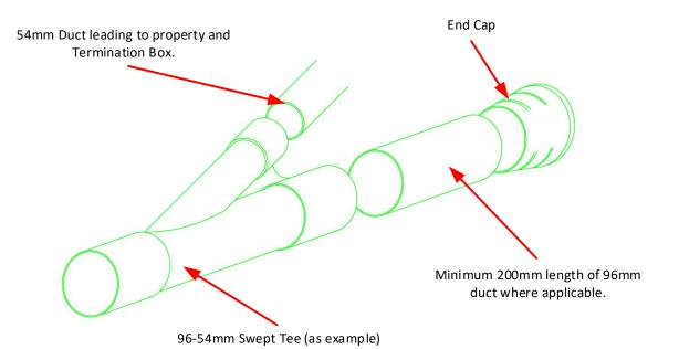
uPVC duct must be cut back before pulling cables externally, this prevents damage to cable while trying to tidy at 2<sup>nd</sup> fix.
