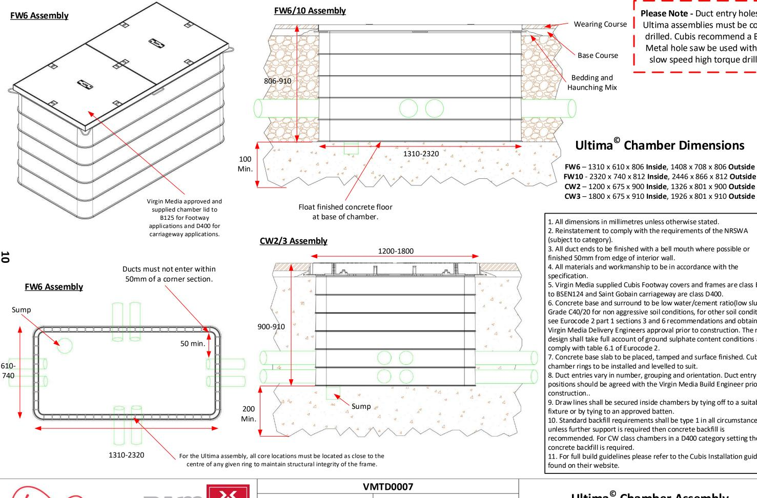
Please Note - Duct entry holes in Ultima assemblies must be core drilled. Cubis recommend a Bi-Metal hole saw be used with a slow speed high torque drill.
