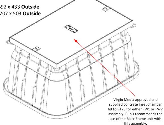
For the Monobox assembly, all core cuts must be at least 50mm from the base of the unit to maintain structural integrity.
