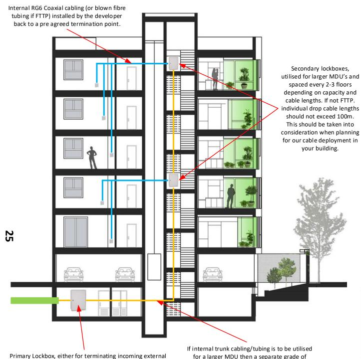
If internal trunk cabling/tubing is to be utilised for a larger MDU then a separate grade of cable/tubing will be supplied which meets the fire regulations required. This can either be installed by your electricians or our cable teams depending on what's easier for your site.
