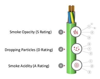
Please note that Scotland has higher standards for the use of internal cabling in high rise units. All Virgin Media supplied cabling is CPR compliant to the highest possible standards.
