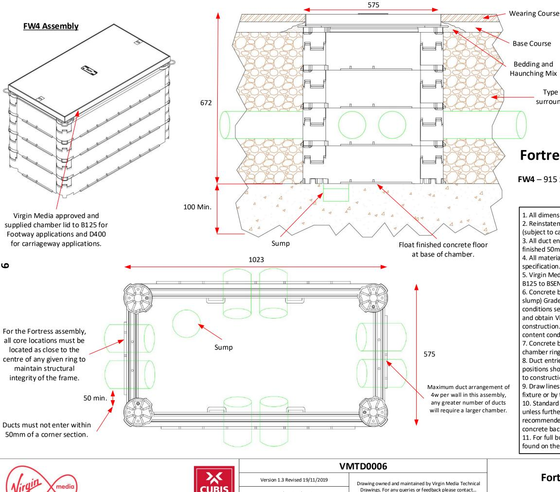
Please Note - Duct entry holes in Fortress assemblies must be core drilled. Cubis recommend a Bi-Metal hole saw be used with a slow speed high torque drill.
